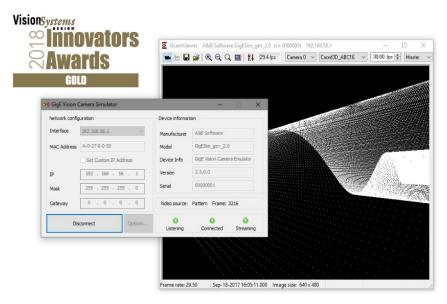
GigSim is a software package that allows end-users and developers to convert their computers, applications and devices into a set of virtual GigE Vision cameras. Any GigE Vision compliant software running at the same or other computers on the network will treat GigESim as an actual GEV camera. GigESim includes a powerful SDK that allows developers to assign images generated by their application to a simulated GigE Vision
